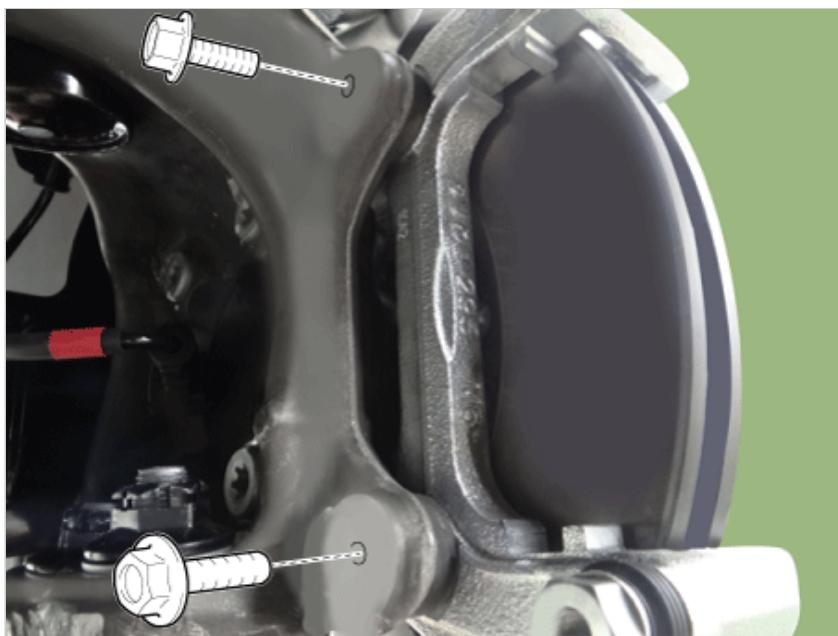
5. Loosen the brake disc screw and then remove the brake disc.
